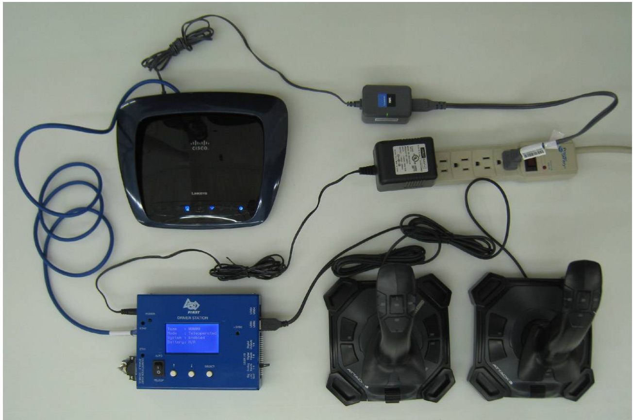
Figure-1.1 Driver Control System with Wireless
